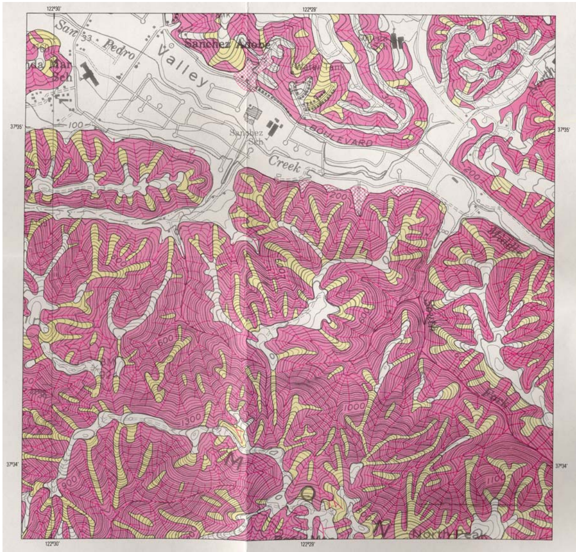
Figure 36c: Debris flow susceptibility map updated from the 1977 version with likely debris flow runout paths (Smith 1988).
